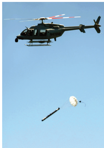
A Bell 407, acting as a surrogate Fire Scout autonomous helicopter, drops a replica torpedo during the ANTX exercise.
